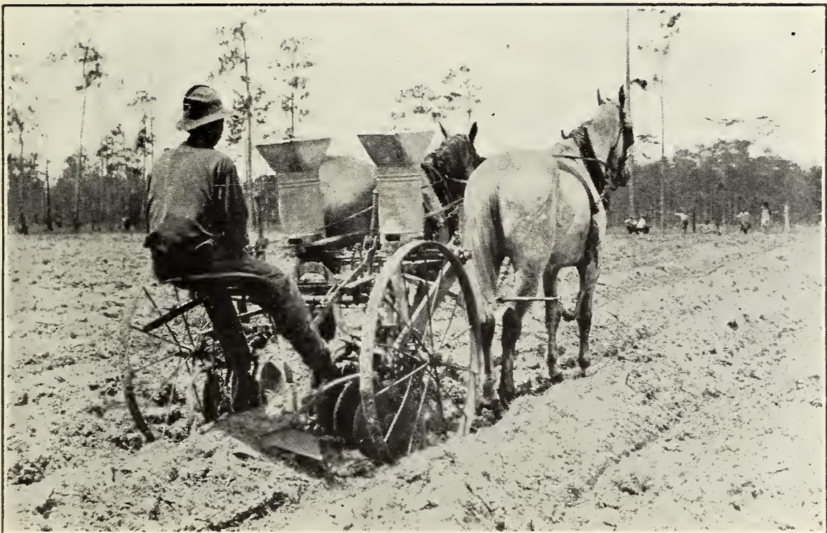
Cultivator distributing fertilizer, making up, smoothing down and center marking beds for planting sweet potatoes—all one operation
