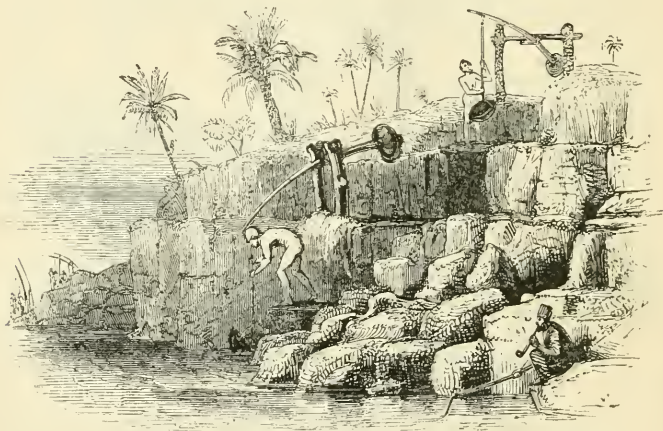
b. Modern shadoof , or pole and bucket, used for raising water, in Upper and Lower Egypt.
